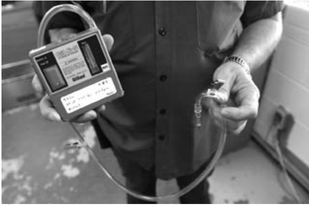
Safety technician Bob Tennant shows an air sampler that must be worn while in certain portions of the Cotter site. Daily Record News Group/Jeff Haller
