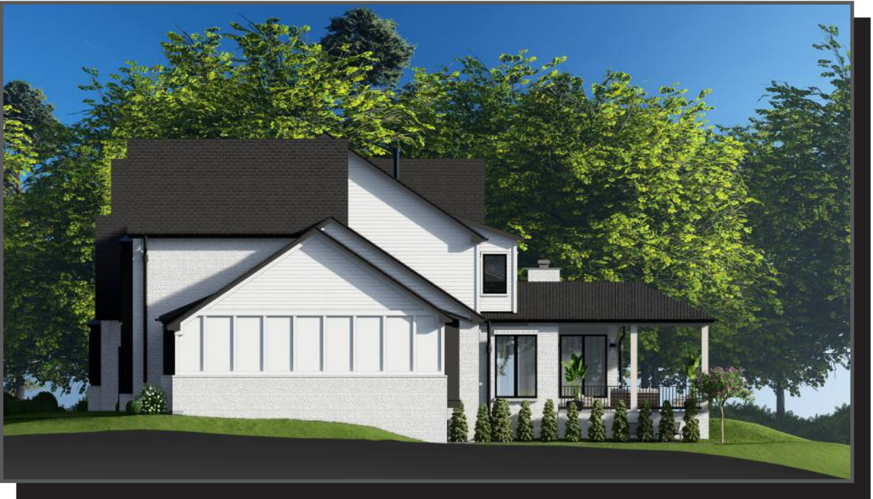
LEFT SIDE ELEVATION SHOWN AS A PARTIAL LOOK-OUT FOUNDATION WITH OPTIONAL WALK-OUT WELL. ALSO SHOWN WITH CUSTOM HEARTHROOM AND COVERED PATIO.
