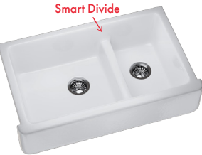
Kohler 6427-0 Min. Cabinet Required: 36" O.D. 35-11/16" x 21-9/16" x 9-5/8" Apron Height: 8-13/16" Cast Iron - White Smart Divide Strainer Basket(s) Not Included Bottom Grids Available
