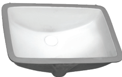
Chemcore TRENCH O.D. 20-7/8" x 14-5/8" x 8-1/4" Bowl Depth: 6-1/4" Colors: White or Bisque Drains Not Included
