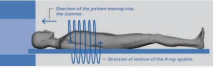
As the table moves through the CT unit, the X-ray system rotates around the patient; images of the body are acquired in "spiral movements".
