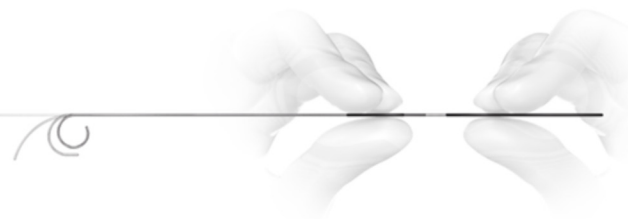
Figure 1 The Drivewire 24 is a novel 0.024 inch steerable guidewire with a deflectable tip controlled via a proximal handle. This allows for in situ, real-time tip deflection.
