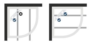
With the unique connect2 design even Quadrant and the Kudos unique Full Curve shape trays have the ability to avoid joists.
