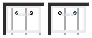
Where joists run parallel to the width of the tray, at least one hole will always be clear.
