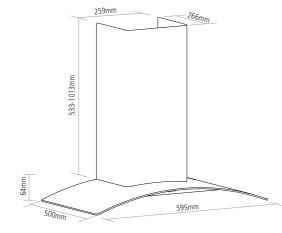
650mm space for electric hobs and 760mm space for gas hobs required from worktop to the mesh filter behind the centre glass panel. From the lowest point of the hood the distance required is 450mm for electric hobs and 550mm for gas hobs.
