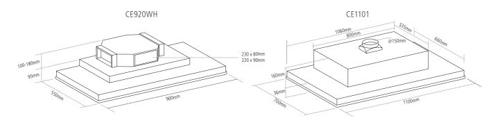
For installation into the ceiling a niche of 865mm by 515mm is required, with a minimum height of 200mm
