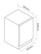
Ventilation requirements - Please allow an 127mm gap around the whole appliance when installed next to a wall, unit or in an alcove
