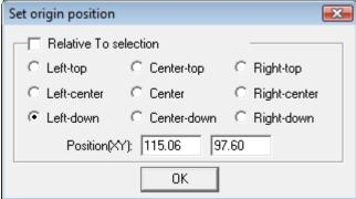
We need to change the "Laser Origin" so that our starting point begins on the bottom left. This allows our new file to align the green markers to the previously cut markers.
