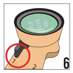
Move lever to 1 and pull handle down until you hear a \*click\* then lift the handle up.
