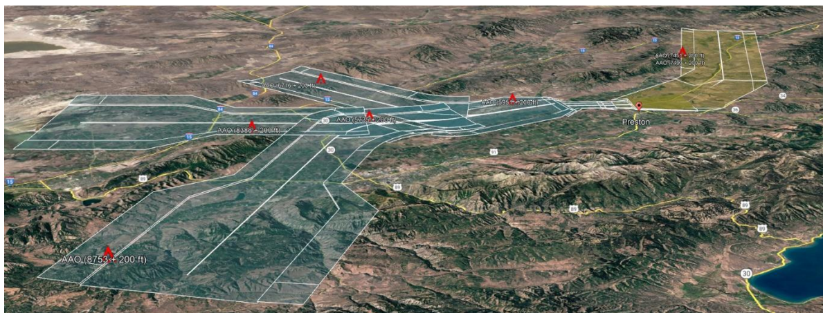
Figure 5: Obstacle Evaluation Areas (OEAs) for Proposed RNAV (GPS) Approach to Runway 4
