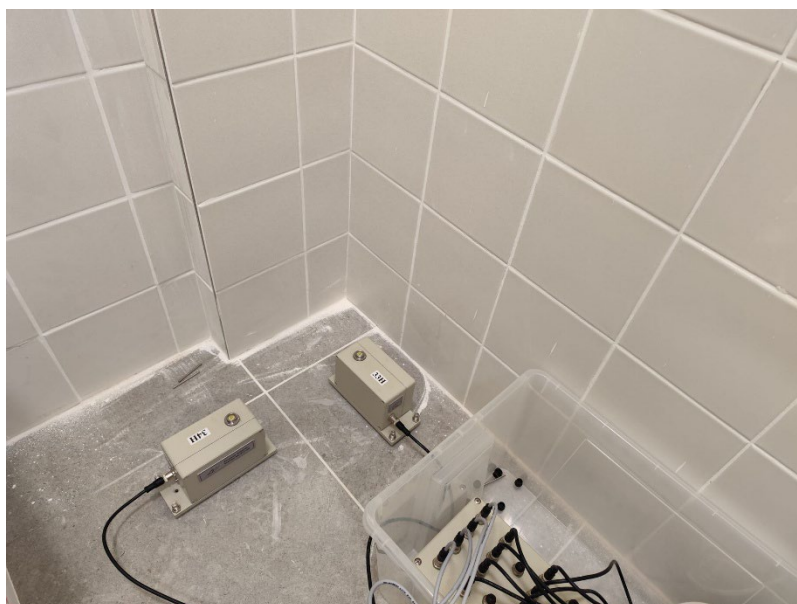
Figure 7.4: A couple of sensors placed near one of the middle columns during the second campaign
