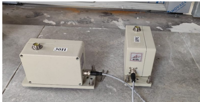
Figure 7.1. The monolithic mechanical seismometer, produced by ADV3S™ and used for the dynamic identification
