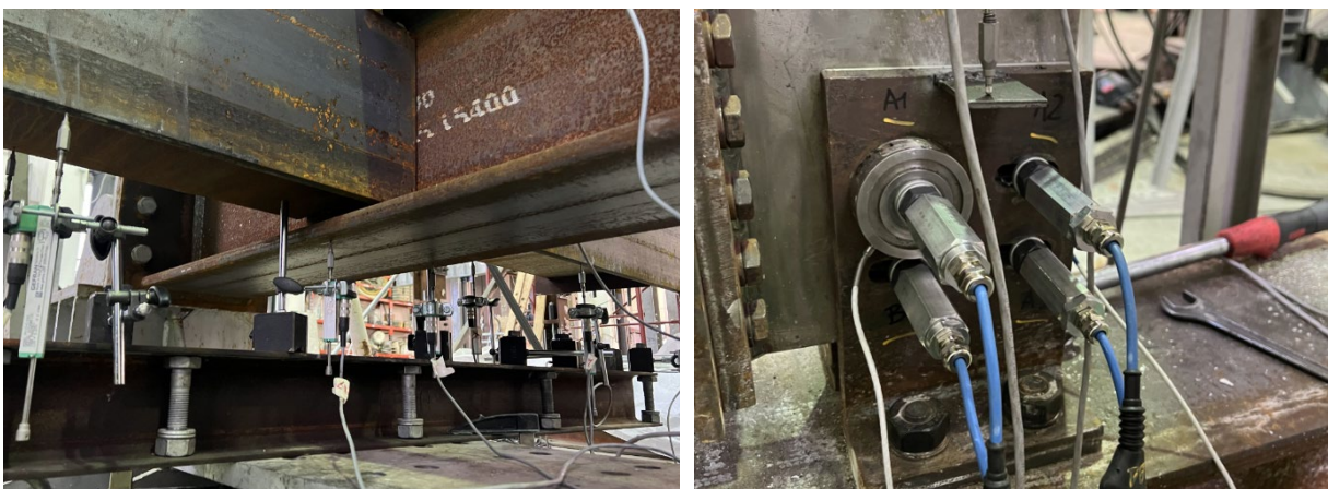
Figure 3.13: Sensors placed on the specimen before the test
