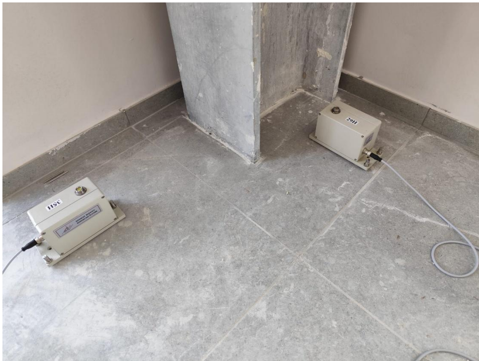
Figure 5. Sensors 29H and 35H in the high left corner of the building with reference to Figure 4
