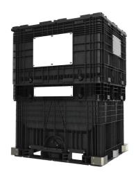
This 57 x 45 x 65 hopper bottom container, with its smooth, funnel-shaped interior, is ideal for controlled dispensing of seed, grain, resins, powders, pellets, and other small components. The adjustable slide gate allows contents to be emptied in as little as 30 seconds. Made from high-density polyethylene, this 2,500 lb.-capacity, collapsible bulk container will provide years of reliable service under the harshest conditions. 100% recyclable. Container lid included. Black color.
