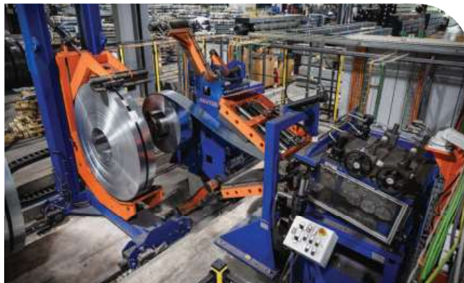
The FCF mill doesn't use round mother tubes to create squares and rectangles, so no material is compressed in the corners, saving users anywhere from 2.5% to 8% on the width of strip used for the tubing.
