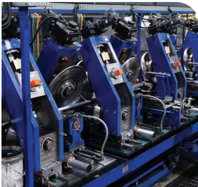
The FCF mill forms square and rectangular tubing directly from strip and from the ID rather than the OD.
