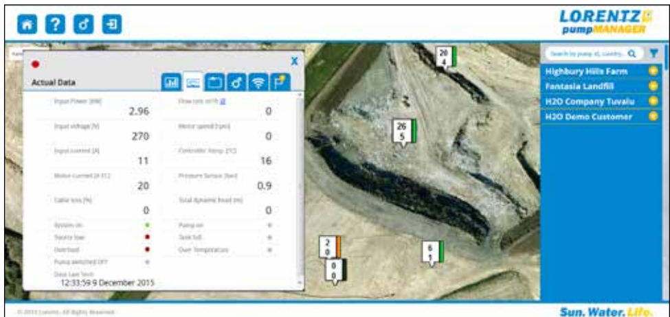
Figure 37: pumpMANAGER view of installation site
