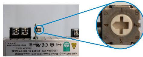
Figure 2: Voltage switch selector
