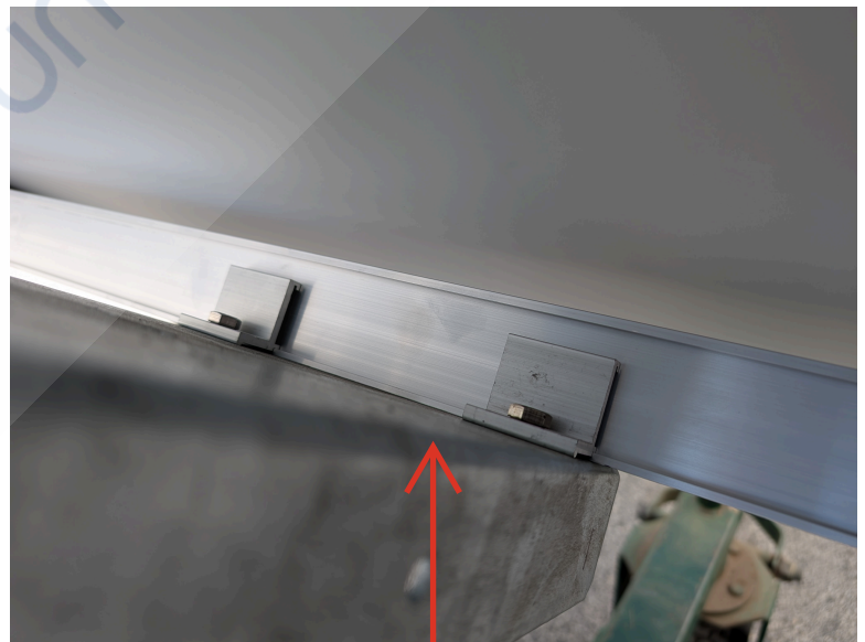
Clamps fixed in position
