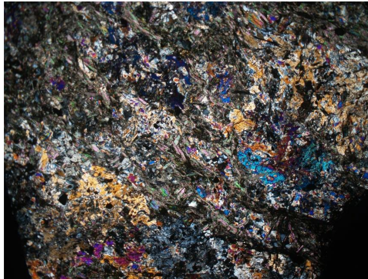
Picture 4: microscopic characteristics of sample 23DM11025 . Polarized light. Field of vision 10mm. Identical shot of picture 3: the section is cut thicker than 30 microns, therefore the general appearance and the interference colors are not the canonical ones of the minerals under analysis. (20I, NX)
