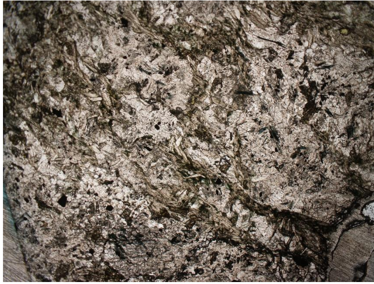
Picture 3: microscopic characteristics of sample 23DM11025 . Parallel light. Field of vision 10mm. The section is cut thicker than 30 microns, therefore the general appearance and the interference colors are not the canonical ones of the minerals under analysis. (20I, N//)
