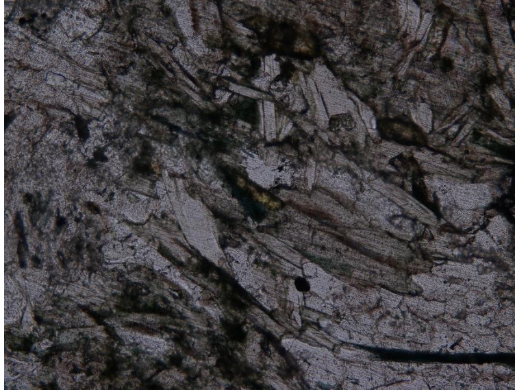
Picture 5: microscopic characteristics of sample 23DM11025 . Parallel light. Field of vision 2 mm. The clearest mineralogical phases are made up of muscovite lacinias. In the center of the image there are two elongated crystals iso-oriented to the muscovite. Below a dark green chlorite lacinia, and just above a yellowish-green pistacitic epidote. The section is cut thicker than 30 microns, therefore the general appearance and the interference colors are not the canonical ones of the minerals in analyses. (100I, N//)
