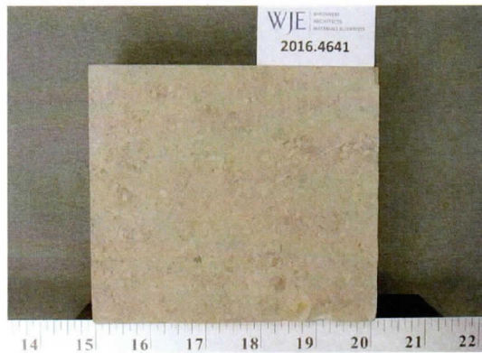
Figure 2. Lapped section cut parallel to the top surface of the sample block.
