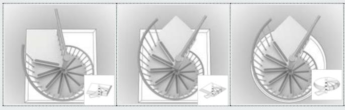
UNIVERSAL LANDING WITH 60° OPENING: adaptable to any opening during installation.
