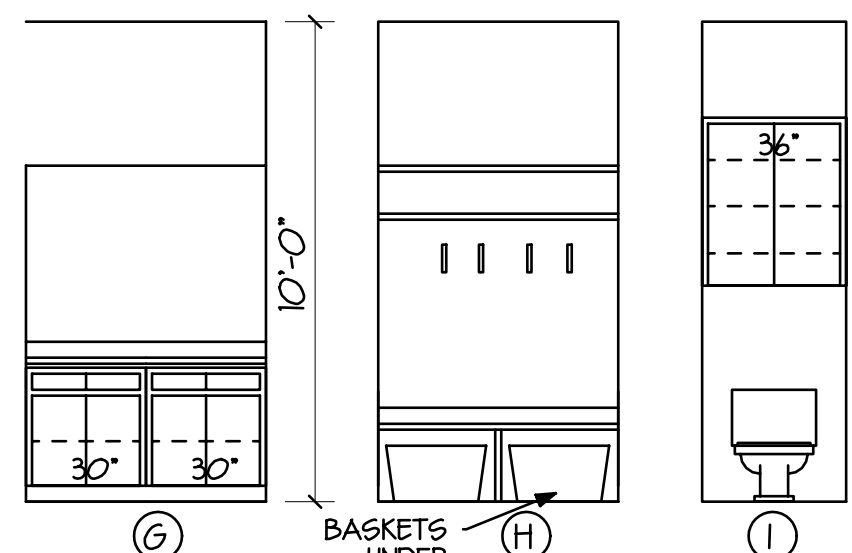
CABINET ELEVATIONS SCALE 1/4" = 1'-0"
