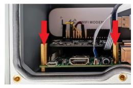
Remove these 2 screws to release the board from the case
