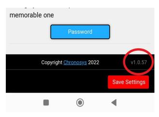
To test you're fully updated, power up your Odin in setup mode. Scroll to the bottom of the UI and you will see the Firmware version number. The number SHOULD match the version number of the file you downloaded.
