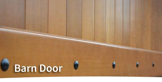
This is the Barn 86mm or 135mm door design. 86mm or 135mm VJ Western Red Cedar is fixed to a Black powder coated frame vertically with 140 x 18mm bullnose Cedar attached horizontally to the door with cup head bolts.
