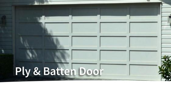
This is the Ply and Batten door design. Ply is fixed to a Black powder coated frame and 12mmx90mm thick cedar border. We use 9mm thick Exterior Marine Grade Ply. Ply is a natural product that has colour and grain variation.
