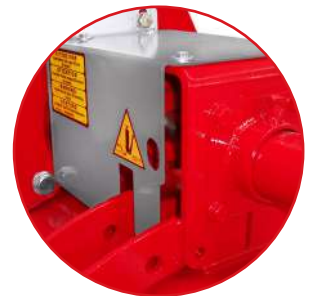
Carter trasmissione Transmission cover
