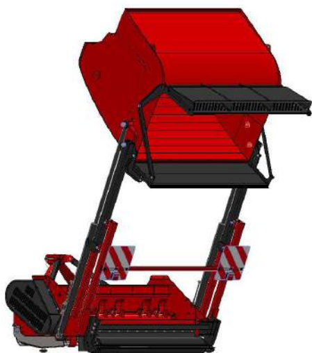
Scarico in quota High unloading system
