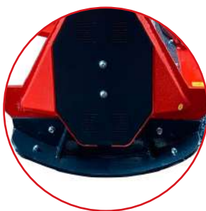
Slitta in hardox Hardox skids
