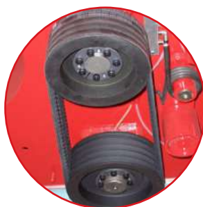
Tendicinghia automatico Automatic belt tightener
