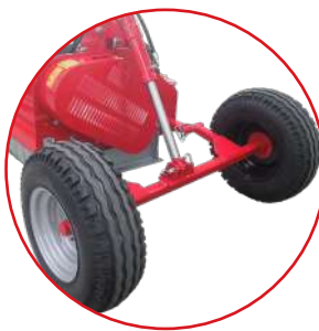
(OPTIONAL) Trasporto idraulico Hydraulic transport
