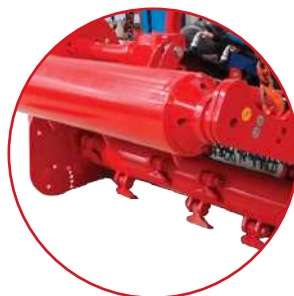
Apertura cofano idraulica Hydraulic hood opening
