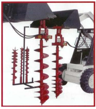
Hub includes sealed bearings. Power unit has a Parker motor and roller chain with speed reduction.
