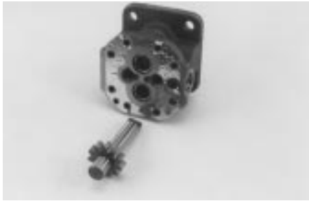
14. Remove the drive gear assembly from the stator.
