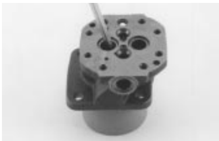
17. Remove the oil seal from the stator, be careful not to mar or scratch the seal bore.
