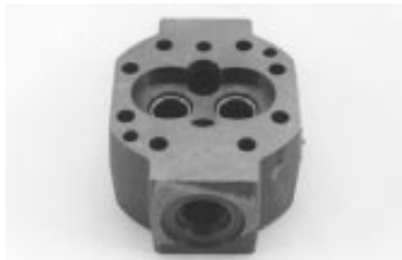
16. Remove the o-ring from the stator.
