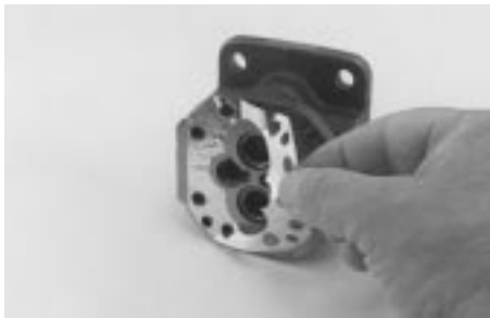
15. Remove the plastic gasket from the stator, this gasket may also remain on the gear housing. (Important! Please note the color of the plastic gasket and use a new gasket of the same color when reassembling the pump).
