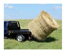
**4** | To raise the bale activate the "**Load**" function on the switch pendant until bale is resting solidly on the flat surface of the Pro Spear.
