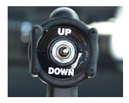
**2** | Utilizing the hand held pendant in the cab of the truck, lower lifting spears to the bottom of their travel by activating the "**Unload**" function on the switch pendant.
