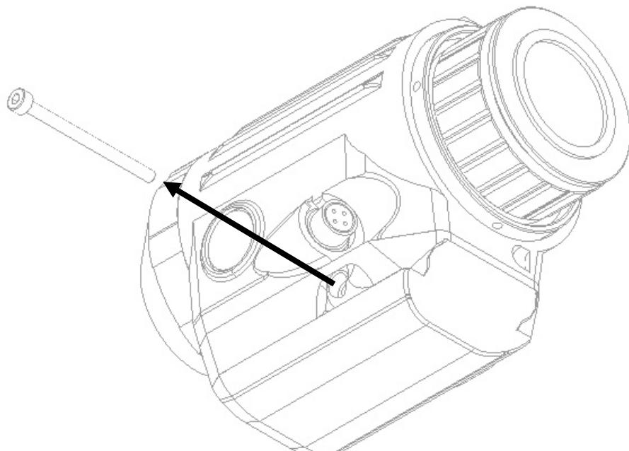
3. Slide the mounted adapter out along the rail to remove it.
