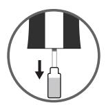
2. Open reservoir, pull down old cartridge to disengage.
