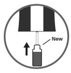
3. Remove protective tube from new replacement cartridge and slide onto long hose attached to notch in iClean PRO.
