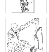
Lift up the scrub deck slowly until it's standing upright on the front wheels; guide the body towards the scrub deck until it snaps into a resting position.
