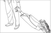
If you would like to load the i-mop into a vehicle or lift it over obstacles, always use two hands. With one hand, hold the pole/handle, and with the other hand, lift the scrub deck.
