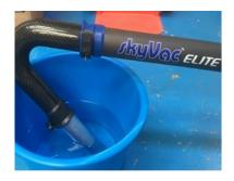
After every shift, flush the inside of tubes and flexi hose by sucking half a bucket of water up into the vacuum and empty. This help keep the pole joints clean from grit.
