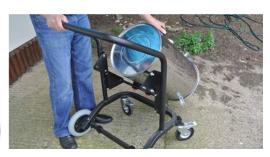
To empty SkyVac remove the head and tilt the bin forward.
