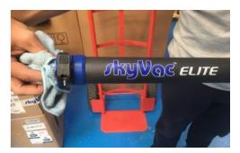
TIP: During cleaning wet or damp gutters, dirt can sometimes stick and line the inside of your poles. The poles will get cold to touch and the weight of the poles will be increased slightly. To remedy this place the end tool in water and suck up a small amount of water.
