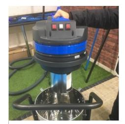
Make sure the switches rest in front of the handle so the deflector plate in front of the filter is in the correct position.
