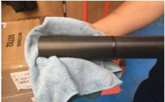
Always clean your poles to ensure the joints are clean and free from grit/dirt which may prematurely wear the joints.
