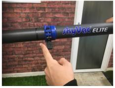
Insert the pole up to the positive stop and no further.
