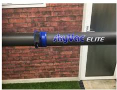
Adjust tension of clamp and close off.
