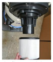
Clean filter on a regular basis. The filter is washable, for best results allow filter to dry before use. Make sure pleats are clear of debris.
