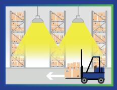
When motion is detected, the sensor will switch on the light up to 100%, or pre set light level preferred by the customer.
