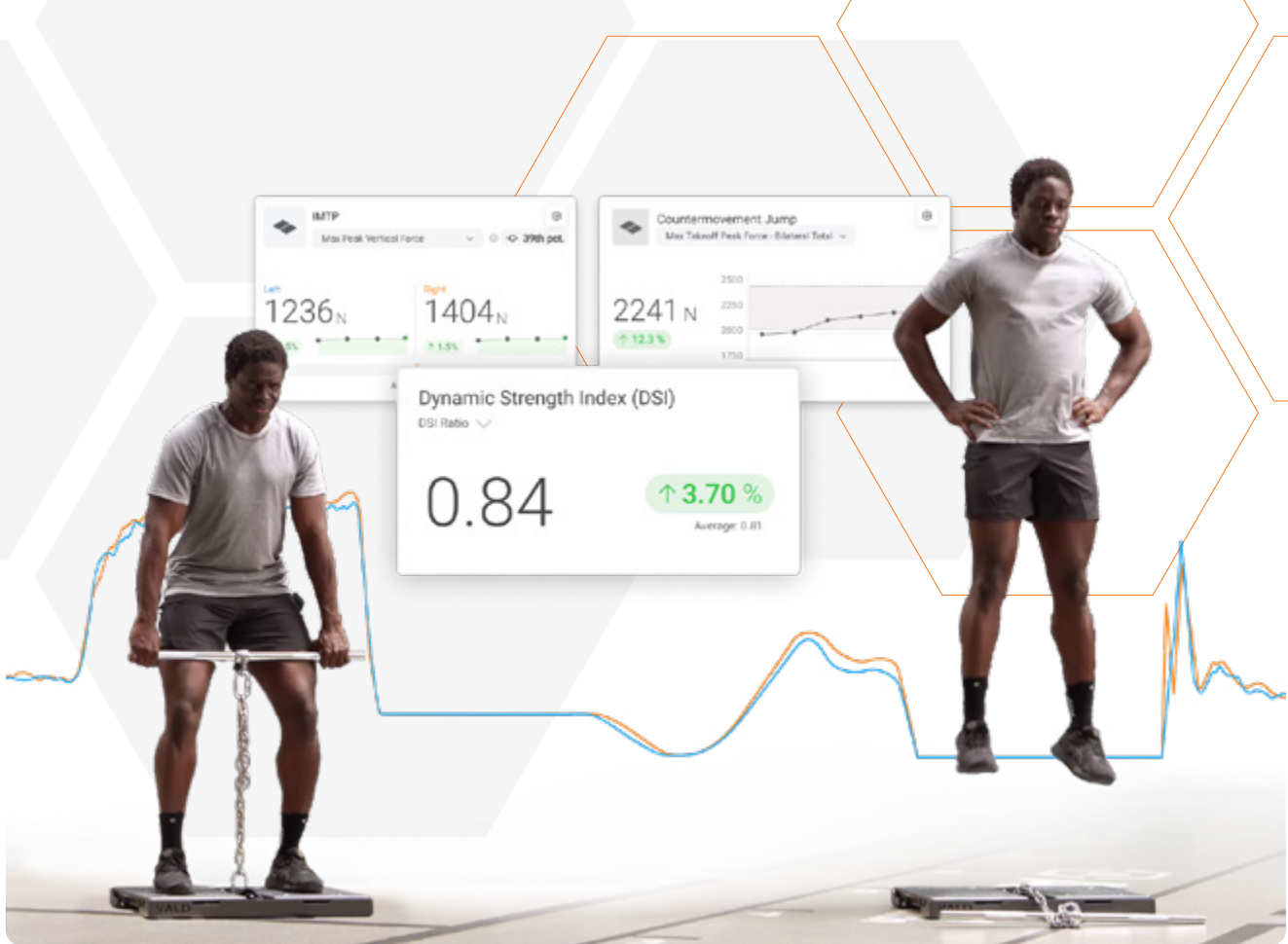
An example DSI result from an athlete performing an IMTP test followed by a CMJ test with ForceDecks.
