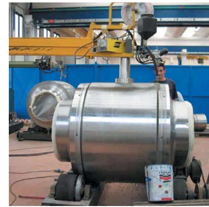
SAW robot welding a 36" Class 600 Valve
