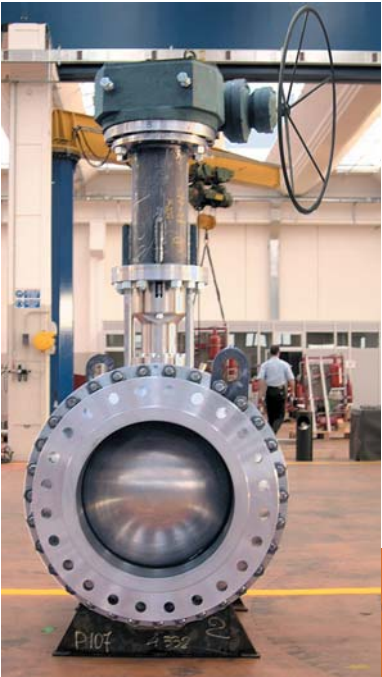
24" (600 mm) class 300 side-entry for high temperature.
