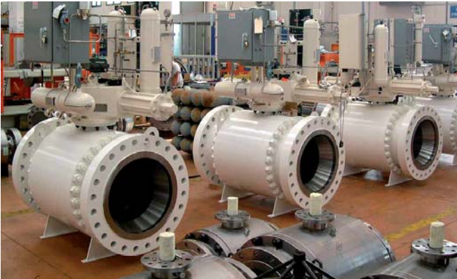
Valves assembled in Valve Automation Center
