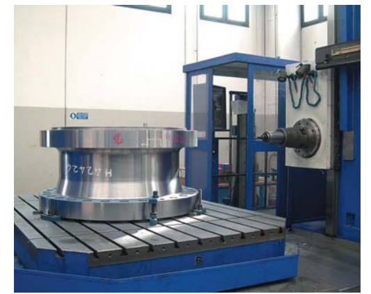
A horizontal boring mill in operation.
