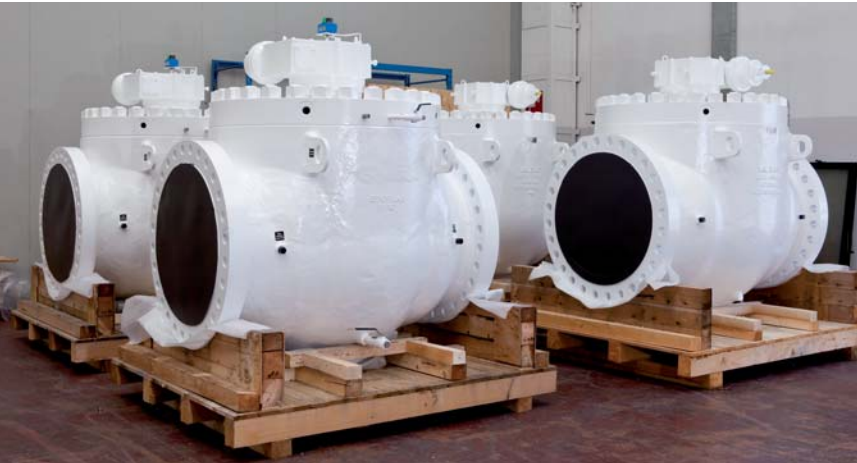
36" (900 mm) class 600 top-entry cast bodies in production.
