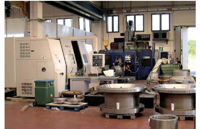
Horizontal (foreground) and vertical (background) lathes.
