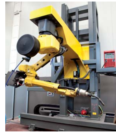
SAW Welding Robot applying weld overlay on valve closure
