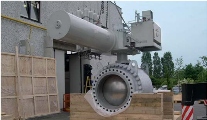
48 inch Class 600 valve with Electrohydraulic actuator
