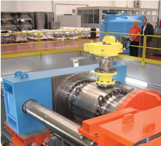
Testing facilities for valves up to 64 inch (1600 mm).
