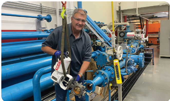
Flowserve engineers conducted numerous hours of cycle testing on the new high-cycle soft seat arrangement before finalizing the design.
