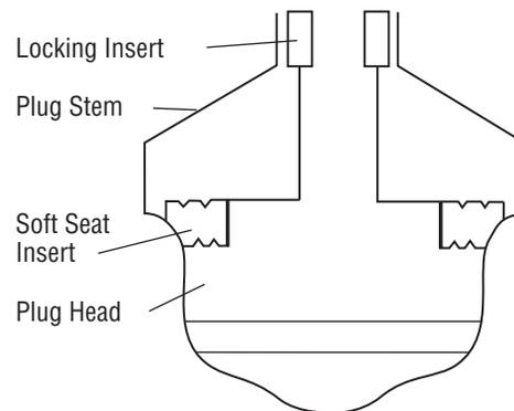
Figure 4: Threaded Plug Head
