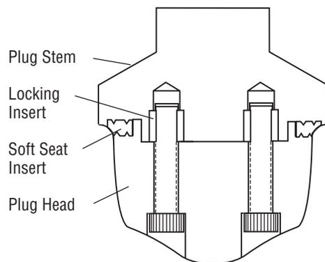
Figure 5: Bolted Plug Head
