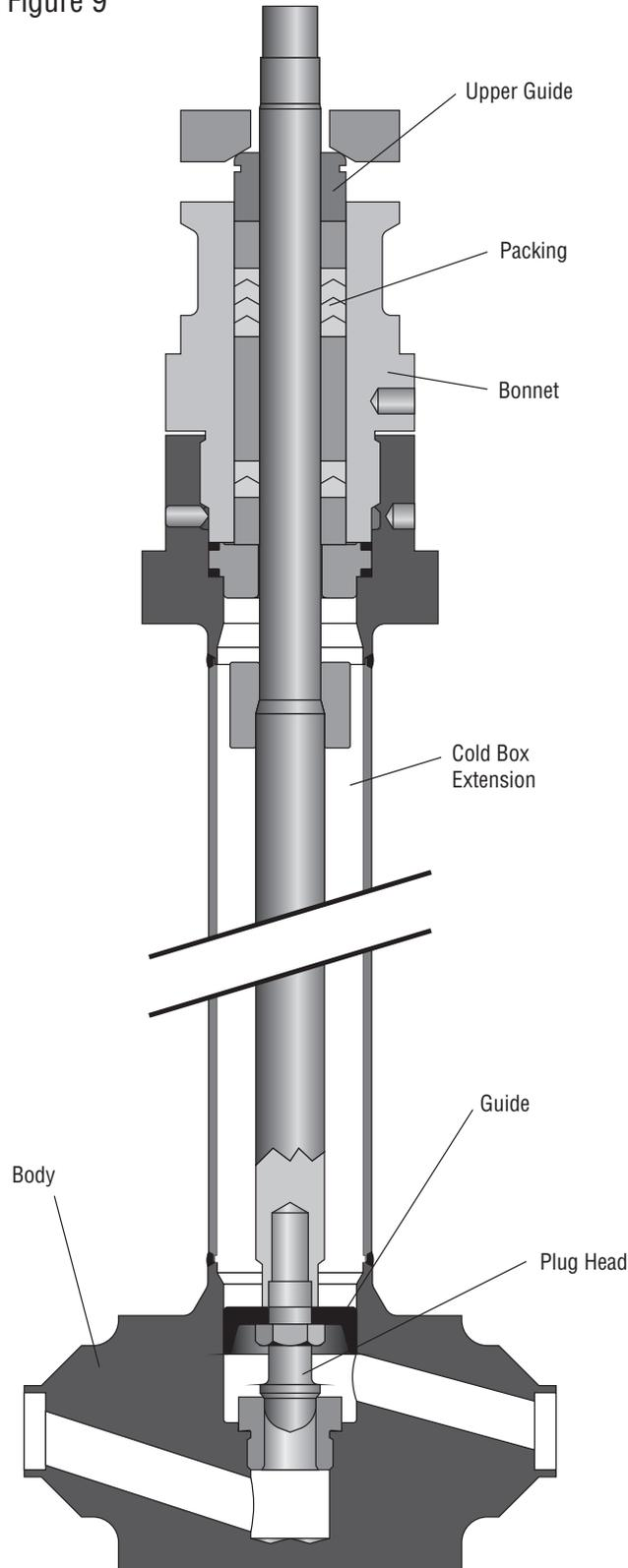
For small, precision flow in cryogenic service, the Mark Six Low Flow is the answer. Using the same principles as the standard Mark Six, the Mark Six Low Flow was redesigned to give precision control over valves with very small capacities. The smallest valve can have a maximum capacity as low as 0.012 Cv.
