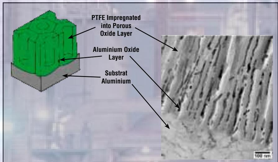
The MaxGuard™ process is applied to the actuator body and both end caps providing an armored layer of protection – both internal and external.
