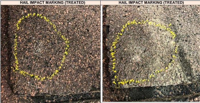
A4. Hail Impact Steel Ball Test per UL 2218 on Treated Material
