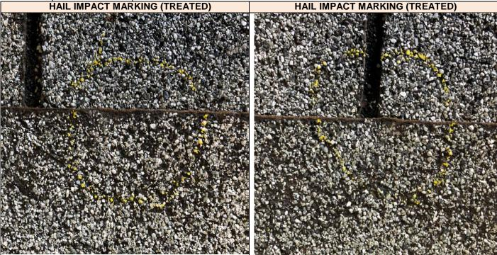
A6 Hail Impact Steel Ball Test per UL 2218 on Treated Material HAIL IMPACT MARKING (TREATED)
