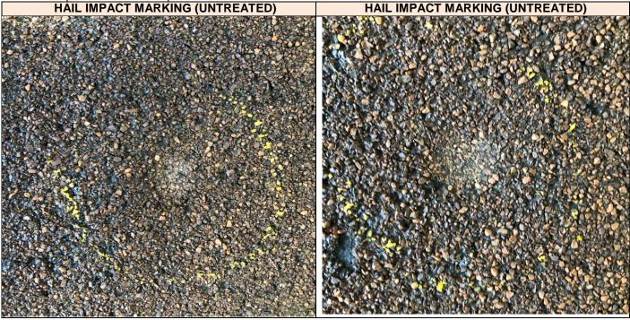
A8 Hail Impact Steel Ball Test per UL 2218 on Untreated Material
