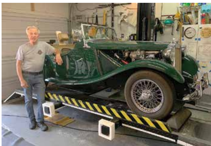
Mort Resnicoff and his 1950 MG TD elevated in his home garage on his single post car lift. Fully raised he can walk under the car comfortably for repairs or upgrades.
