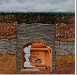
Air pressure inside an inverted glass will not allow the water level to rise more than a fraction of an inch. Perhaps you have seen this effect in your kitchen sink. A Clark Grave Vault protects its contents using the same principle. Its dome-shaped design allows air pressure to build, keeping moisture out.
