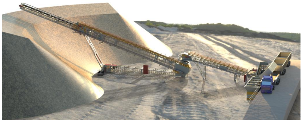
TITAN Side Tip - Bulk Reception Feeder feeding 20m Fixed Link Conveyor feeding TS 52 Radial Telescopic Stockpiling Conveyor, Stockpiling Material.
