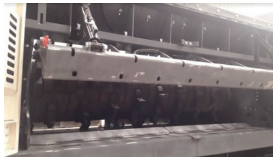
Hydraulically operated access doors on both sides of the chamber for teeth replacement and servicing
