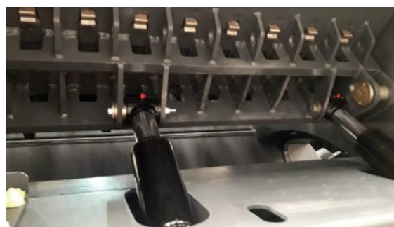
Hydraulically adjusted counter comb allowing product size to be altered to requirements
