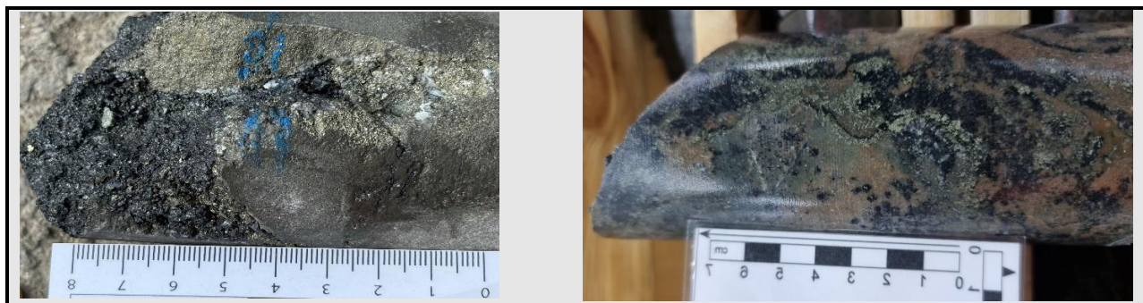
EL24016_60.6m Enargite, chalcopyrite and pyrite cementing diorite fragments
