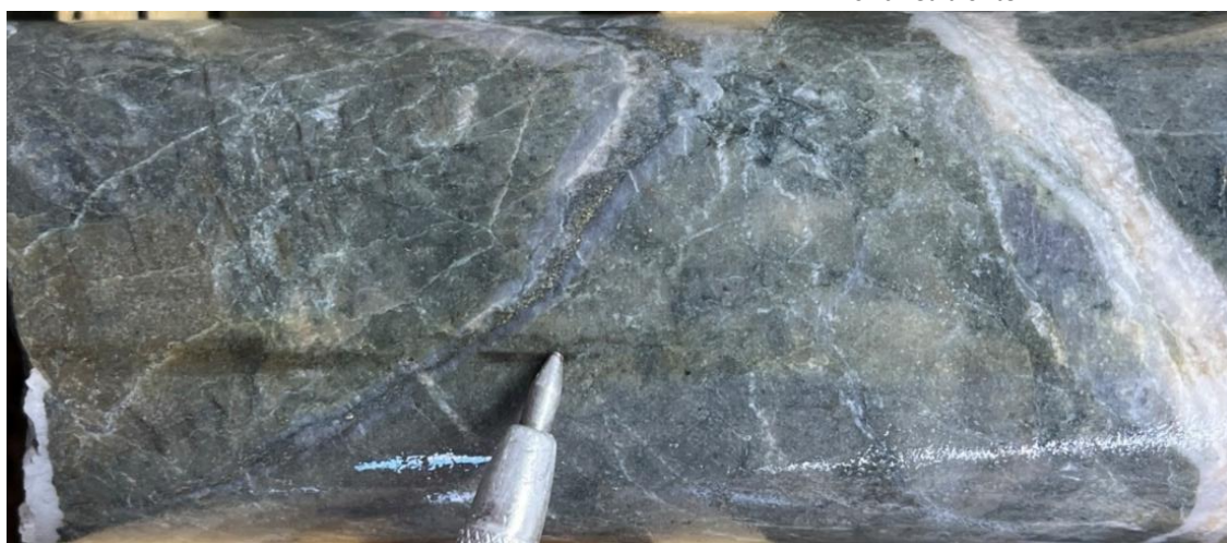
EL25012_465.1 m B-vein - Quartz vein with pyrite and chalcopyrite along centreline of quartz vein
