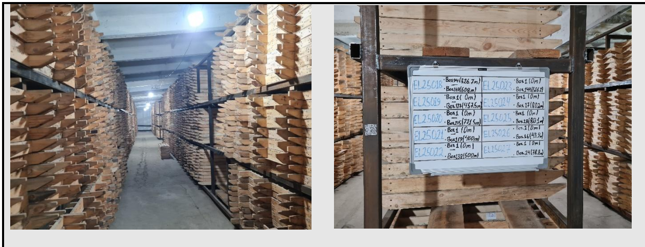
Figure 45. Ekidos LLP storage facility with Elemes core, with labelling and QR codes identify holes and intervals stored in each section, located in Ekibastuz, Kazakhstan.
