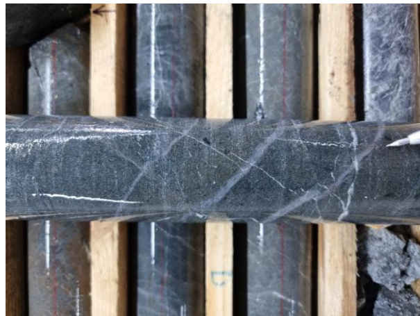
EL24005_533.0m Quartz-pyrite-chalcopyrite veins
