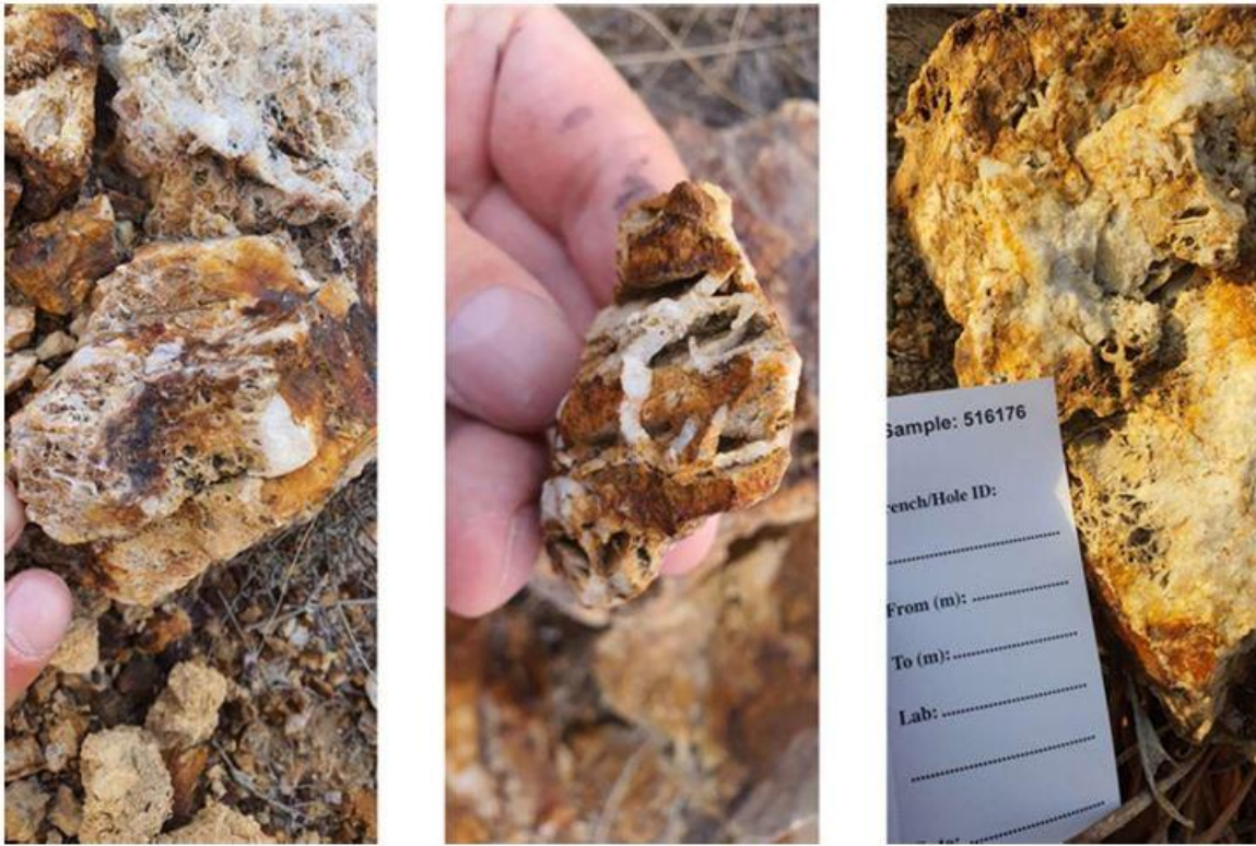
Figure 21. Quartz bladed textures in the surface rock chip samples from the K-Ozek project on Elemes license
