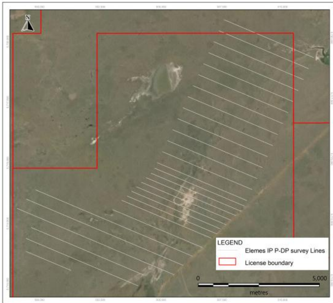
Figure 31. Location map of the planned IP survey lines over Berezski mineralization trend
