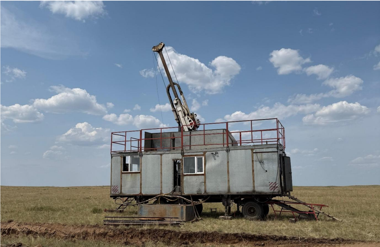
Figure 40: Iskander ZBO Drill Industries ZBO-S15 drill-rig with surrounding drill shack mounted on a trailer bed.
