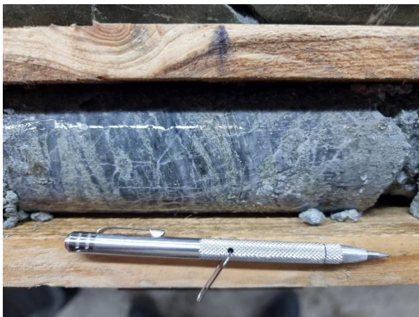
EL24005_536.9m Sheeted quartz-pyrite-chalcopyrite veins
