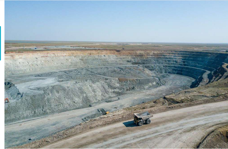
Nearby Bozshakol Copper Mine (produces >100,000 tpa Cu)
