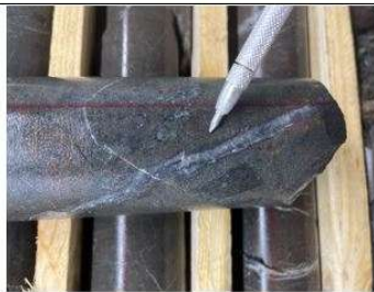
EL24004_128.0 m, Quartz-Magnetite-Chalcopyrite vein, magnetite salvage.
