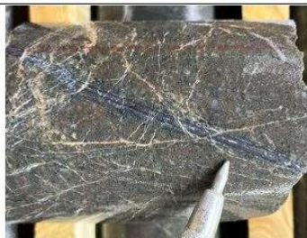
EL24004_304.8 m, Qtz-Py-Cpy vein, with magnetite central suture.
