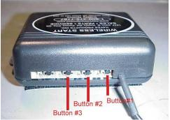
Step 2. Press and hold program button #1 down until LED lights up and flashes.
