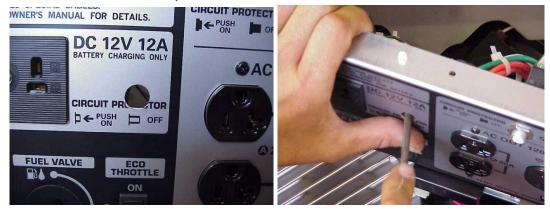
Remove the washer and ON/Off plate from the toggle switch from the WSK-1 harness and mount the toggle switch as shown.
