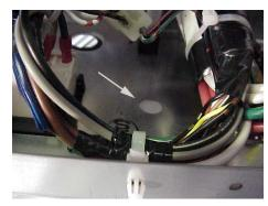
Cut out the front panel sticker from the hole then using a small file, round out the flat portion at the bottom of the hole.
