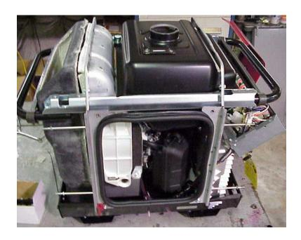
Thread wire harness from WSK-1 remote to back side of control panel from the engine compartment through hole as shown below. Run Black wires from remote under the control panel to the battery.
