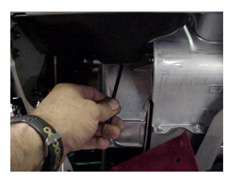
Attach cable holder by removing the adhesive backing and attaching as shown.
