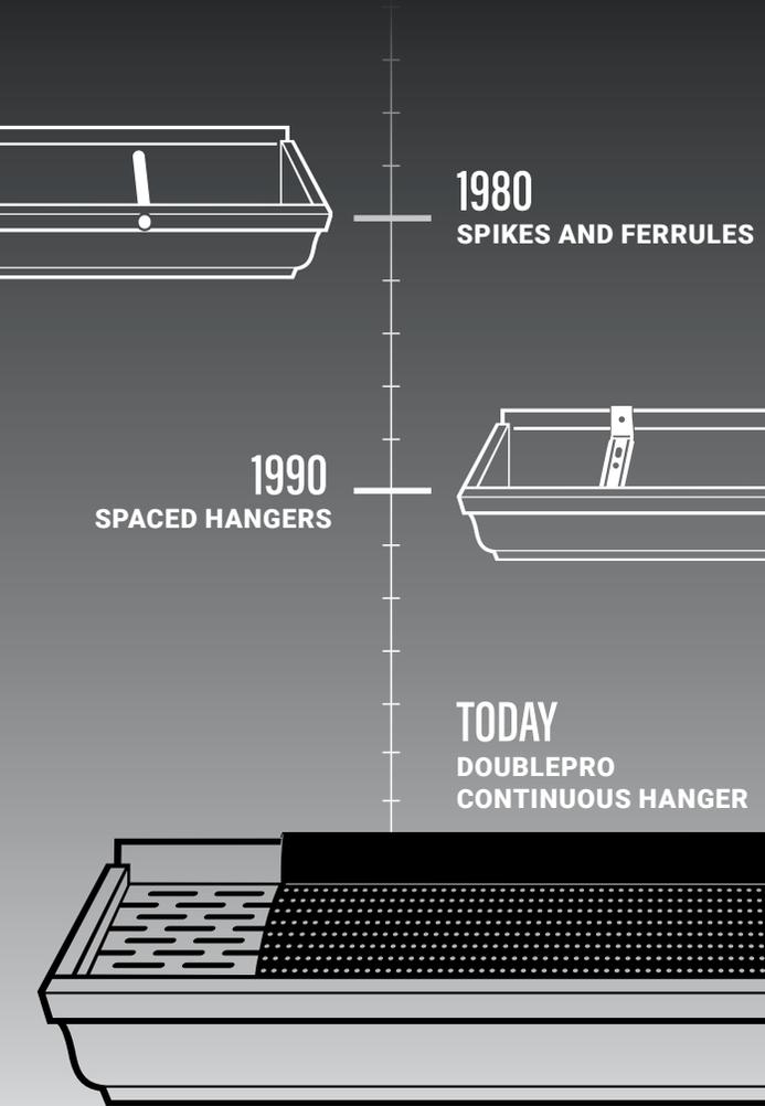
The continuous hanger is the only fastening system that leaves gutters strong and rigid along their entire length. It eliminates the weaknesses that other systems generate between nails and spaced hangers.
