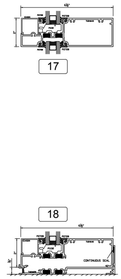
**TUBELITE THERMAL PAIR OF DOORS w/ TU24650 FRAMING**
