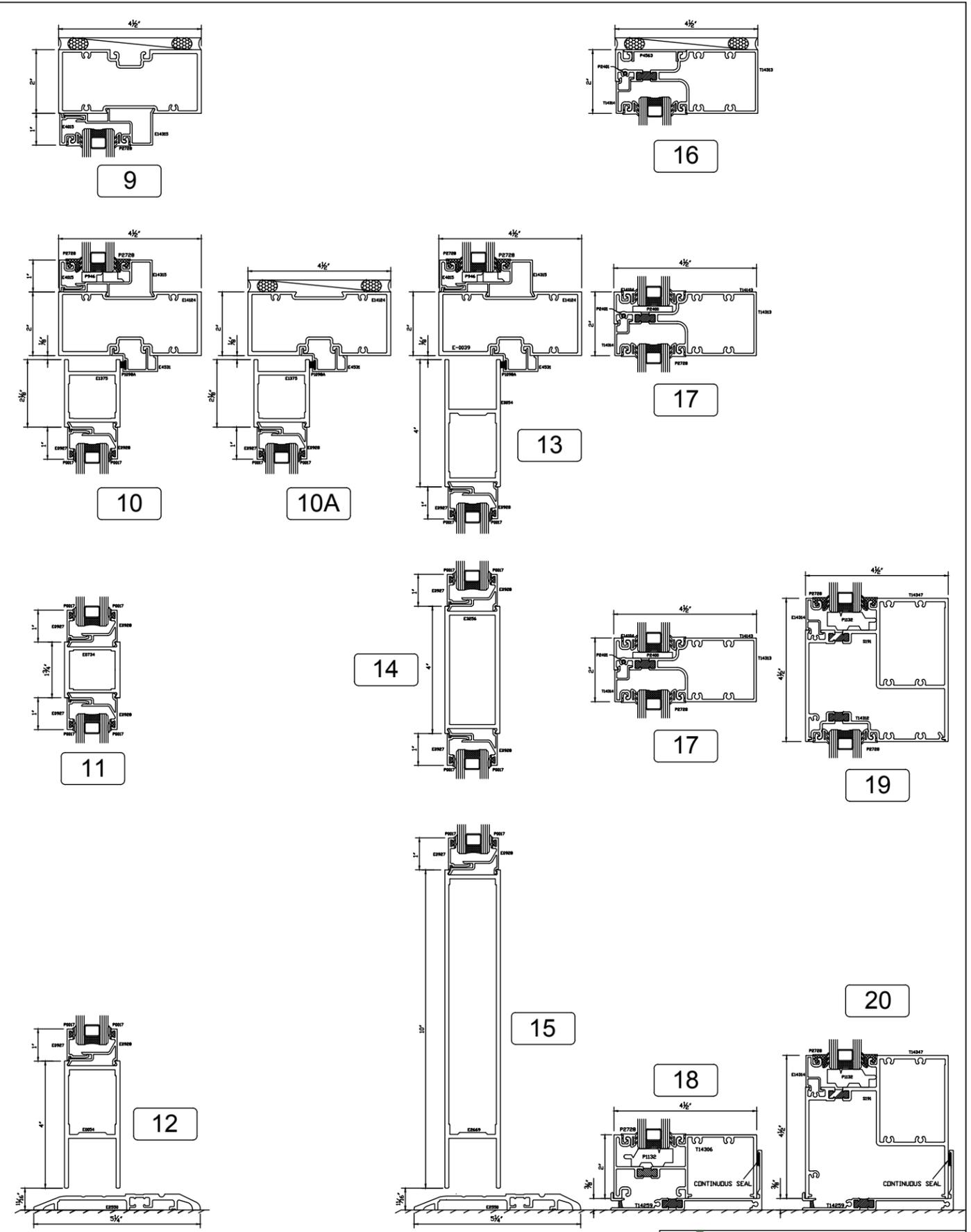
**TUBELITE PAIR OF DOORS w/ T14000-IO FRAMING**
